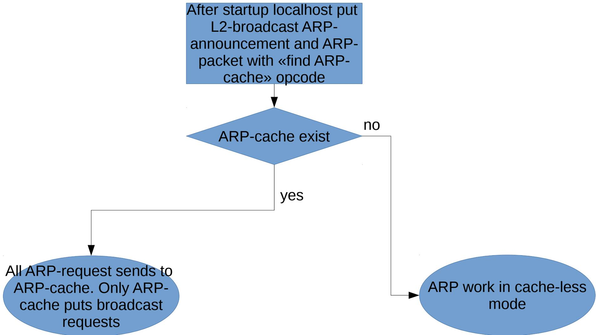
ARP-cache collect MAC-addresses from own broadcast investigations, from ARP-invites, optionally from router searches. Hence you must use local router or L3-switch as ARP-cache for performance hit.
